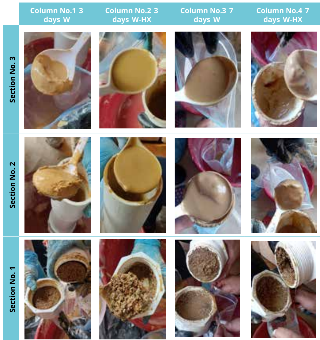
Figure 4. Visual Identification of the Diatomaceous Soil Phases Sedimented in the Columns
